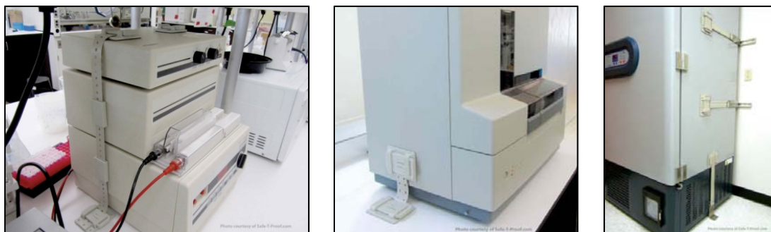
Figure 3. Photographs showing secured laboratory equipment (photos provided by Safe-T-Proof).
