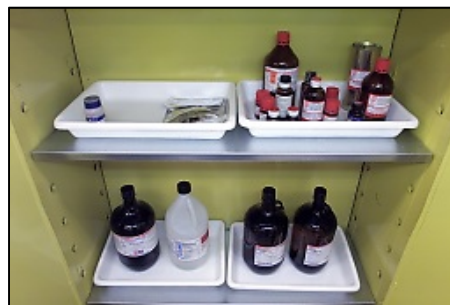
Figure 4. Chemical storage areas showing use of shelf restraints and secondary containment tubs.
