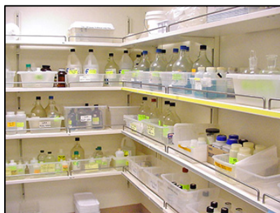
Figure 4. Chemical storage areas showing use of shelf restraints and secondary containment tubs.
